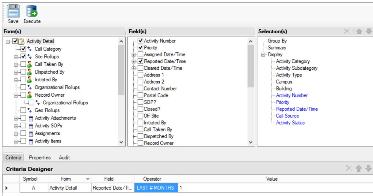
Figure 1 – The **Create New Query** window with activity display data selected.
